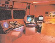
The Marine Institute's Navigation and Blind Pilotage Simulator trains mariners to navigate a vessel safely in restricted visibility with the use of instruments only. *Photo courtesy of the Marine Institute*.
