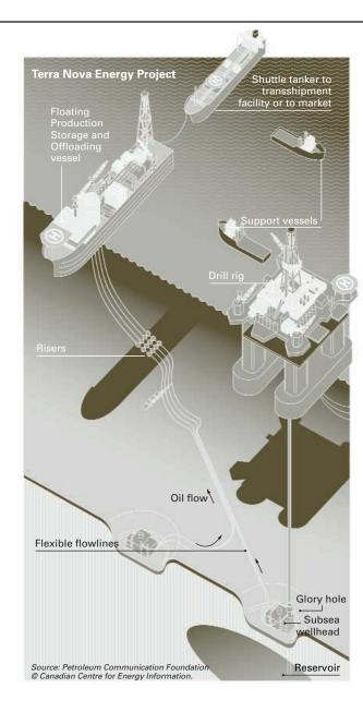
more than 40 kilometres of flexible flowline is used to convey hydrocarbons to and from the wells. Produced gases are separated from the oil and re-injected into the reservoir for possible future extraction.
