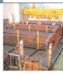
Various types of marine riser and drilling pipe are stockpiled aboard an offshore platform. *Photo courtesy of Ocean Rig.*
