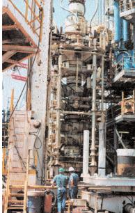
A series of blowout preventers, linked together in a "BOP stack," are used to control pressure while wells are being drilled. Valves in the preventers can shut down fluid circulation quickly and safely in the event of an emergency or an unexpected encounter with high-pressure crude oil or natural gas. *Photo courtesy* of EnCana Corporation.
