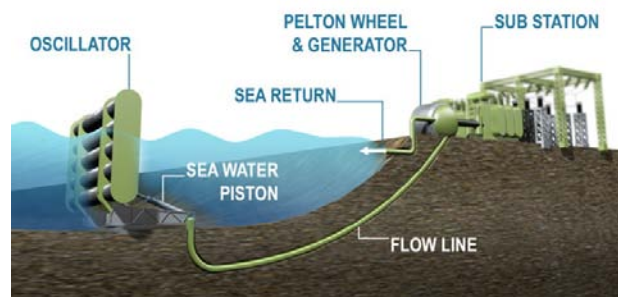
Figure 2.8: An “Inverted Pendulum” wave energy device employing a pressurized hydraulics power take-off system [28]
