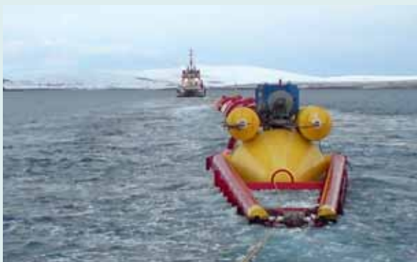
Figure 21 Installation and connection component development for the Pelamis device.
